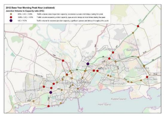
Figure 2.3 Volume / Capacity Ratios at Junctions (2012)
